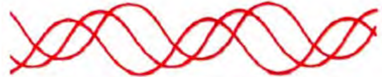
LED: one color (monochromatic) and waves not in phase (non-coherent)
